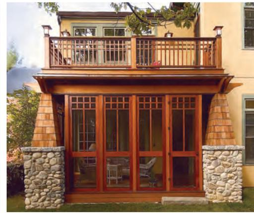
The Woodway Architectural Deckrail Series features pre-assembled railing panels in five patterns. Each pattern is manufactured using mortise and tenon joinery and is secured with urethane glue. The panels are available in net 68 1/2" and 92 1/2" fixed lengths to fit 3 1/2" posts measured on 6' and 8' centers. In a normal installation the finished rail height is over 36".
