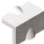
ROLLFORMED CORNER CAP OPTIONAL (USUALLY MITERED)
