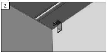
2. Position the clip on the outside of the rim joist securing it with a single screw inserted perpendicular to the joist. After positioning the last deck board in place, secure it by angling a screw through the clip and into the board at a 30°- 45° angle. Be careful to make sure the screw inserts fully and pulls the board down (3). Space no more than 12" (30 cm) apart.
