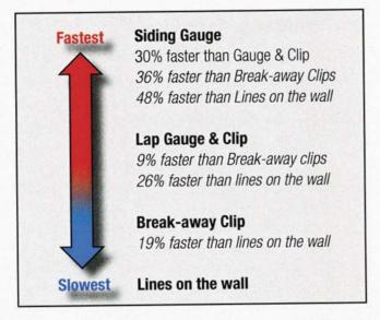
A line on the wall was a very time consuming process and required very precise measurements. To be most effective, it required two people to create the line. Lines can be used at different points on the wall to ensure the siding is level but should not be used as the primary alignment device.
