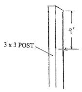
NOTE: If you are using double 2x6's for headers instead of the 3x8's, the mark should be  $7\frac{1}{2}$ " from the top.
