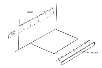
C. Align the rafter hanger on the center of the marks on the ledger board or the wall/fascia with the bottom of the hanger on the chalk line. Install the top screw and tighten loosely. Use a bubble level to straighten the bracket and install/tighten the bottom screw. Completely tighten the top screw. Do this for all of the rafter hangers.
