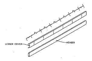
B. (WITHOUT LEDGER) Identify the attaching height on the wall or fascia and snap a level chalk line. Identify and mark the width of the cover on this line. Using a straight edge, place marks above the chalk line at 24" on center. The
