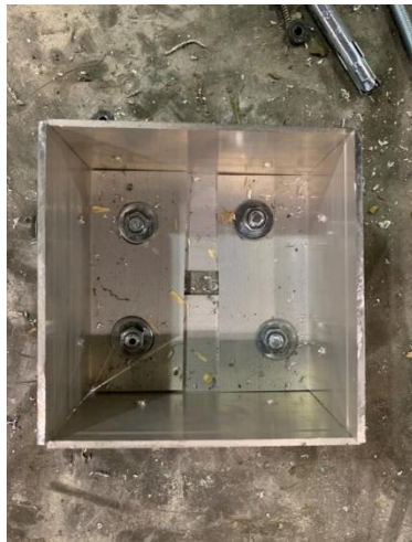
Example of a bottom post bracket made using post scraps cut into four L brackets.
